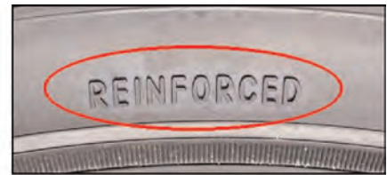
Figure 1. “Reinforced” marking on sidewall.
