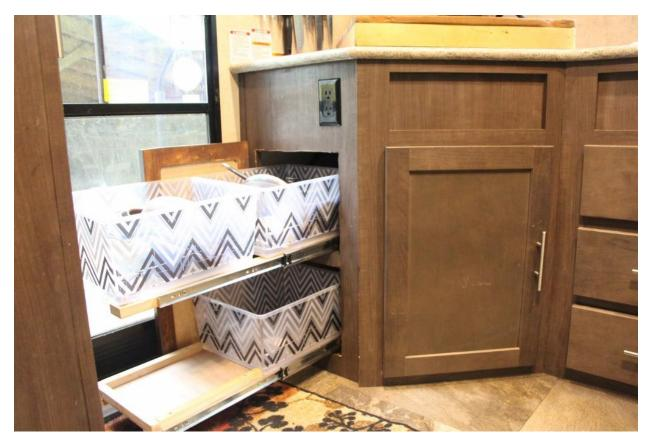
The most disappointing part of the project was the stain I used on the frame. It was a pretty close match to the Pod's finish (vinyl coating) when I tested it on a scrap of the wood I used. However, it didn't react the same when I applied it to the sanded wood of the frame. I may look for some contact paper to match the vinyl coating of the Pod's woodwork.
